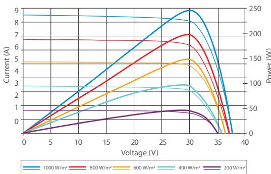
Excellent performance under weak light conditions: at an irradiation intensity of 200 W/m<sup>2</sup> (AM 1.5, 25 °C), 96% or higher of the STC efficiency (1000 W/m<sup>2</sup>) is achieved.
